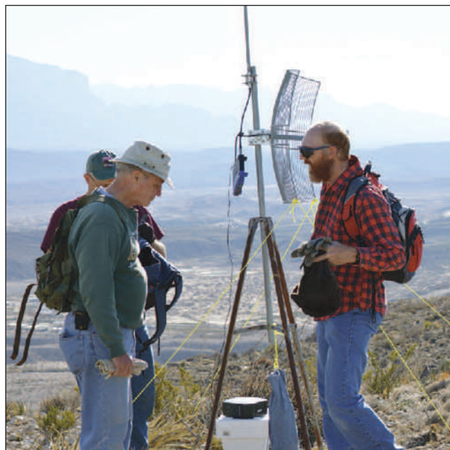
Figure 2 — From the left are Mitch, KD5HCV; Joe, KC2KG, and Alan, KE5DTR, who used a compass to aim the antenna and a signal mirror to confirm the orientation. The antenna is secured with guy wires attached to 10 inch steel spikes. The cooler is to keep the battery-powered UPS warm during the night. [Paul Kinney, KD5VRU, photo]
