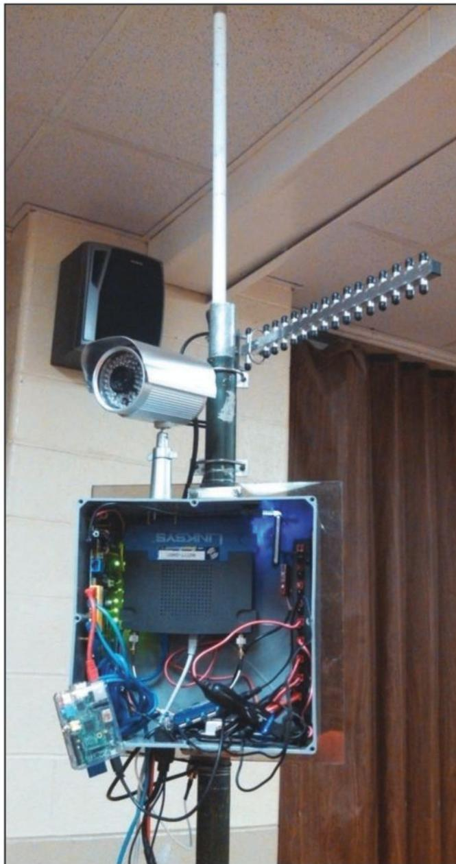
Photo D— The author’s “super node” in progress. When completed, it included an autonomous video camera, Raspberry Pi Server, and an Internet gateway.
