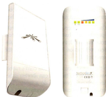
Front and rear views of the Ubiquiti NanoStation Loco router. Available for about $50, all you have to do is load new firmware to turn it into a 2.4 GHz HSM mesh transceiver.
