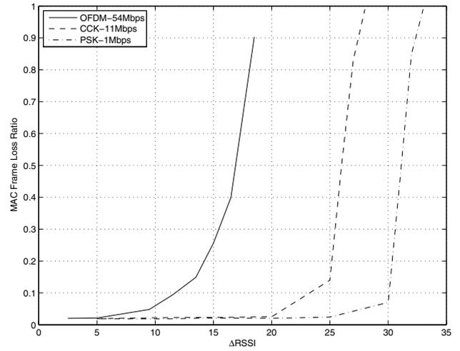
Fig. 9. Frame loss ratio vs.  $\Delta$ RSSI for different modulation schemes.
