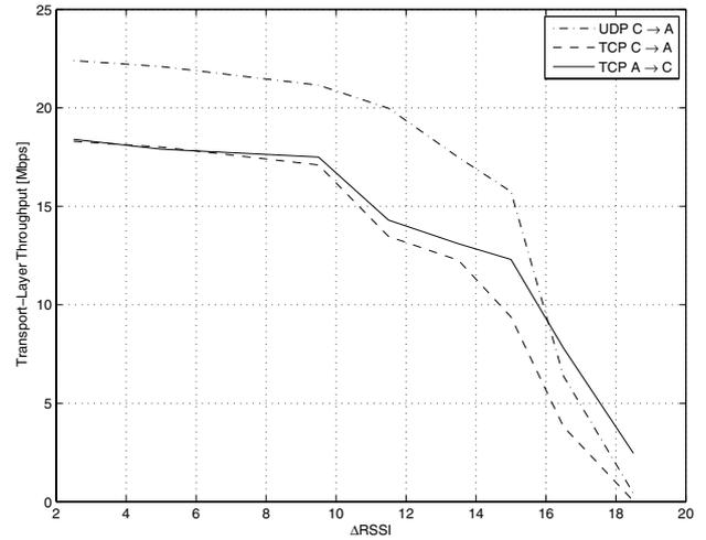
Fig. 11. Transport-Layer throughput vs.  $\Delta$ RSSI using different transport protocols for OFDM 54Mbps.
