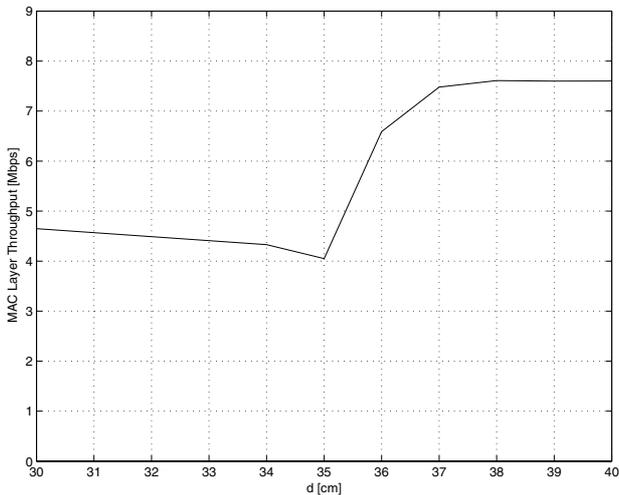
Fig. 5. MAC throughput vs. node distance for nodes broadcasting in channel 3 and 8.
