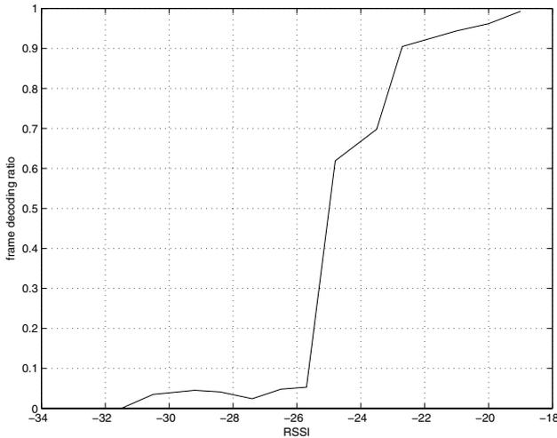
Fig. 8. Ratio of successfully decoded frames vs. RSSI.
