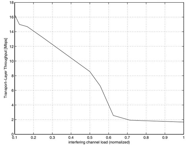
Fig. 12. Transport-Layer throughput vs. normalized channel-load using OFDM 54Mbps.
