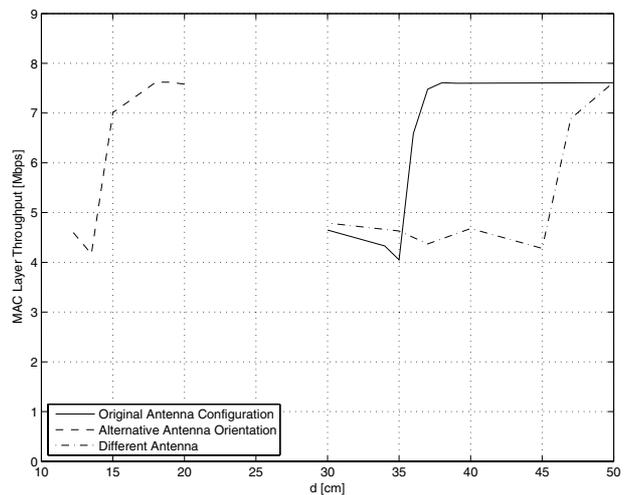
Fig. 6. MAC throughput vs. node distance for three different antennae configurations.
