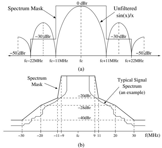
Fig. 2. IEEE802.11 spectrum mask for 802.11b (a) and 802.11g (b).
