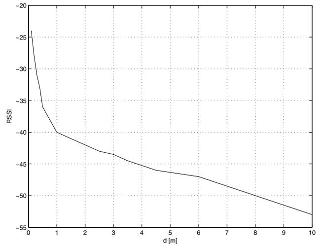
Fig. 4. Averaged RSSI vs. physical distance between node A and B.
