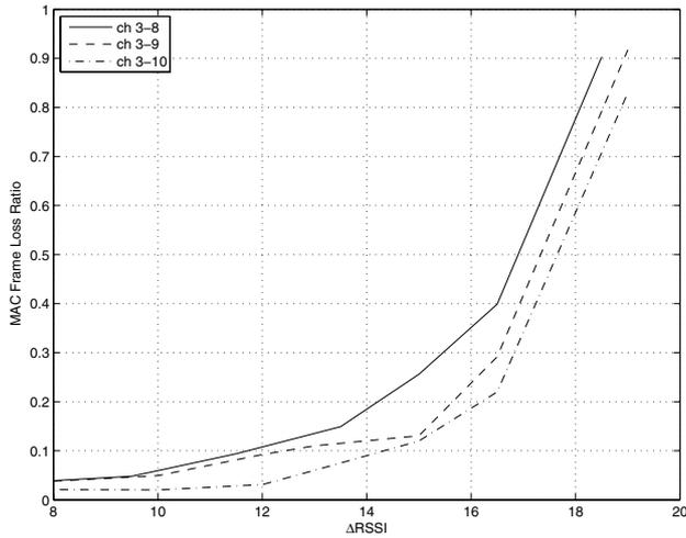
Fig. 10. Frame loss ratio vs.  $\Delta$ RSSI varying the channel separation using OFDM 54Mbps.
