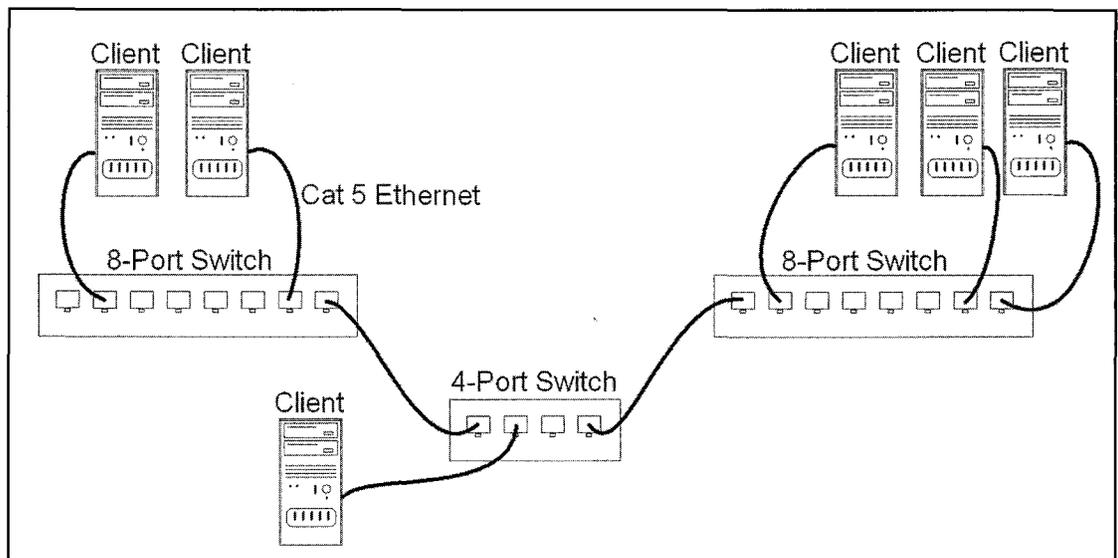
Fig. 1— A typical wired network, with a 4-port switch as its center and two 8-port switches to connect up to 16 client computers (only six are shown for simplicity) together in a wired Local Area Network, or LAN.
